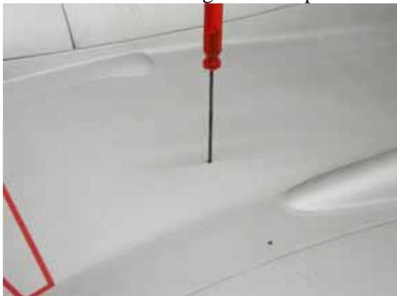
The outer wing panels can now be installed connecting the aileron servo lead, outer flap servo lead, air brake servo lead, and the two main gear door air cylinder hoses. The spars are slid in to the slots and are also secured with (4) set screws per side with a 2mm hex allen wrench, again use care not to back these set screws too far out as reinstallation is difficult.
