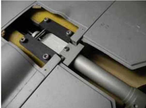
Install the main gear retract assembly to the fuselage with supplied M4x30mm screws, air lines must be fitted to the retract cylinder prior to installing the retract unit as they are not accessible later. The strut cover upper mounting bracket is to be installed at this time, use of thread lock on this screw recommended at this time.
