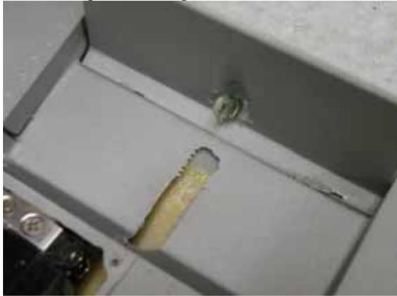
A clearance slot for the control linkage is also cut at this time, it must extend forward and up the wall to provide vertical travel as the servo arm rotates.
