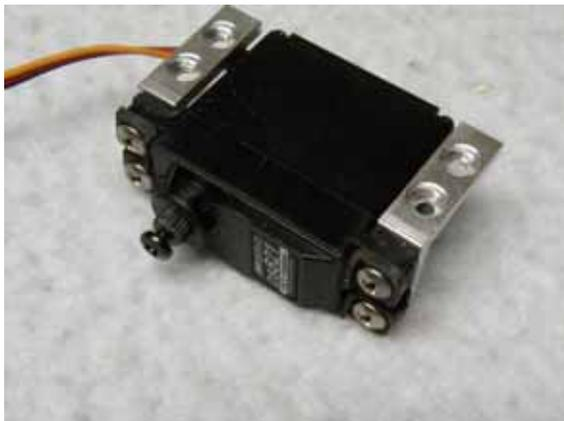
Prepare the servo for installation by mounting the servo on the supplied aluminum angle brackets with M3x8mm bolts. (Use of a JR8611 or equivalent servo is recommended for the elevator servo). Center the servo with the radio unit and install the servo arm. The servo is now
