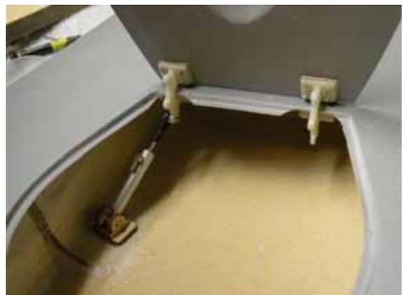
Scuff the inner fiberglass surface and epoxy the air cylinder mount in position.
