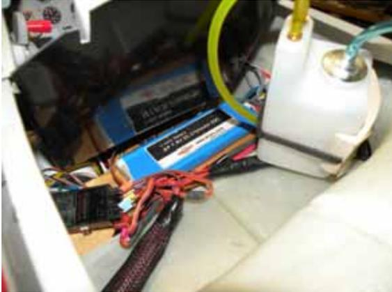
The area behind the cockpit provides for convenient installation of the receiver and ECU battery on the receiver tray board. The receiver battery on the prototype is an A123 2cell 2300 mah battery secured with Velcro between the gun ports and the air tanks.
