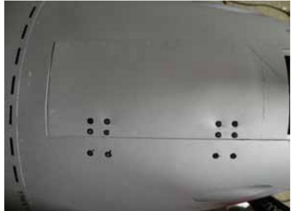
The nose gear door is installed with the supplied offset hinges. Pockets are located on the gear door itself for properly locating the offset hinges. Locate the screw holes as required to assure a flush fit of the door when closed. Assure adequate hinge clearance to fully open the door to clear the nose gear strut and tire, adjust as necessary.
