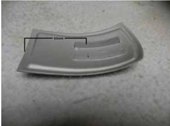
Drill (2) holes 63mm from back edge of the nose gear front cover for attachment to the nose gear cover link rods. Install the supplied fiberglass bracket to the door for installation of the cover closer spring. Locate the nose gear front cover spring tab and epoxy between the link rods.
