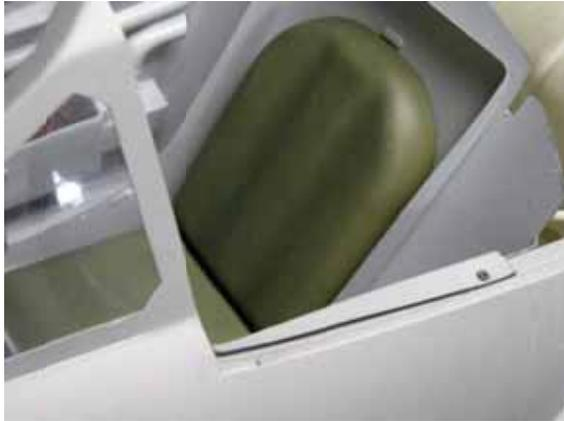
Install the cockpit pit by positioning forward until the instrument panel is forward ahead of the windshield so the top of the instrument panel is hidden, some trimming of the plastic cockpit pit may be required in the area of the windshield frame to position correctly. The cockpit pit is then secured with a small sheet metal screw along the cockpit rails to maintain the forward position of the cockpit.
