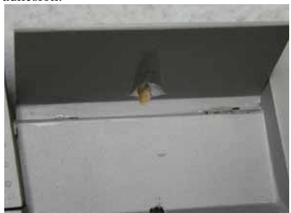
A slot is cut on the inside of the air brake slightly off center in the tunnel for the control horn, care must be taken to not damage the out skin of the air brake when
