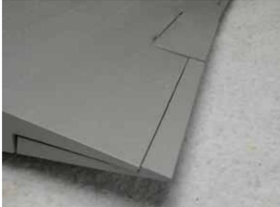
slots as required to obtain a good flush fit of the air brake to the wing panel skin, pay particular attention to the fit on the top surfaces as this is the most observed area of the aircraft at rest. Once a satisfactory fit is made, lubricate the hinge pins and epoxy the hinges in place to both the wing panel and air brake, use care to maintain accurate alignment as the epoxy cures.
