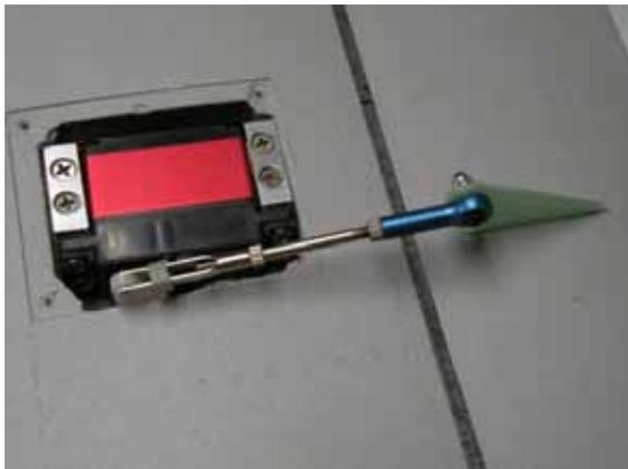
This is the a photo of the final installation of the elevator servo, control horn, and control linkage, with the servo hatch removed to show installation details.
