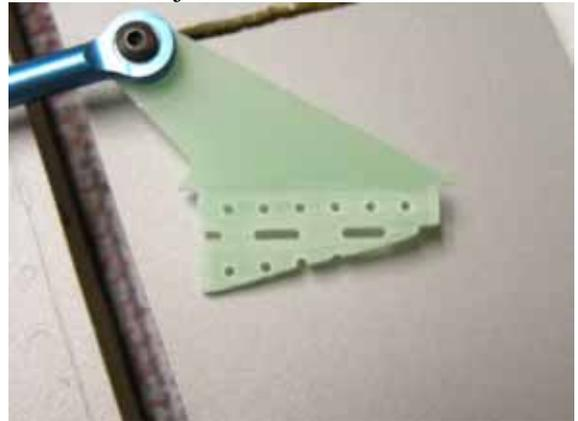
The pivot hole will need to be drilled out for the M3 linkage screw with a 3mm dia. drill bit, a 1/8" dia. drill bit can be used to provide clearance for the M3 screw. Assemble the linkage to the control horn. Rough sand the lower area of the control horn to improve epoxy adhesion.
