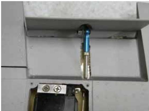
Adjust the air brake for 70 degrees open travel position in the open position.
