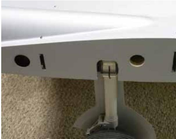
The mating servo lead routing holes should be cut in to the wing center section rib at this time.
