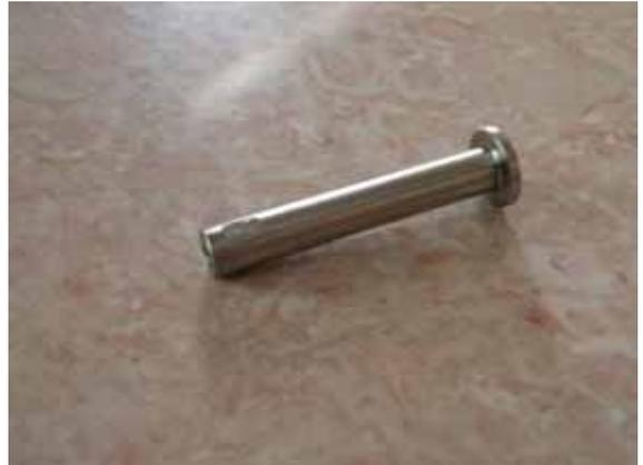
Remove the wheels from the main gear at this time for final setup of gear. The axles will need flats ground on them for contact by the retaining screw. While the wheels are off remove the wheel half retaining screws and apply threadlocker then tighten these screws in a circular pattern to assure a tight grip on the tire.
