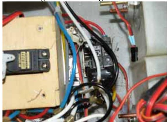
The landing gear retract servo and valve and a double solenoid valve for gear doors was mounted behind the nose gear steering servo. Note the mounts must be installed to allow removal to maintain clearance for removal of the main fuel tanks.
