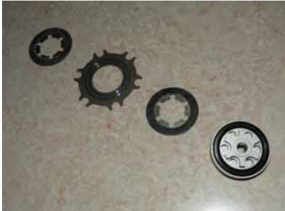
The brake components are shown for illustration purposes to aide in reassembly. The double sided brake pad is on the far left, then the brake disk, the single sided brake pad, and the brake caliber on the right.
