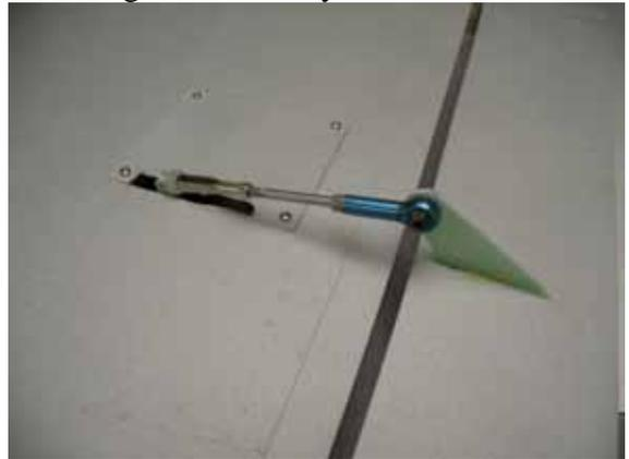
Note the control horn for the aileron will again need to be trimmed to attain a flush fit.
