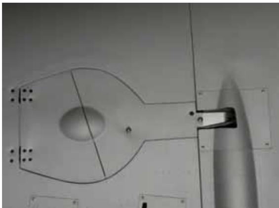
At this time locate the gear strut cover in the door pocket, measure location of lower attach screw and drill hole for mounting screw. Attach the door with the lower mounting screw. Position the gear door in the pocket and drill and tap the upper strut mounting bracket and secure the strut cover at the top end. Scrap plywood shims will be required to assure proper fitting of the door to the wing skin. Once properly fitted secure the screws with threadlocker.
