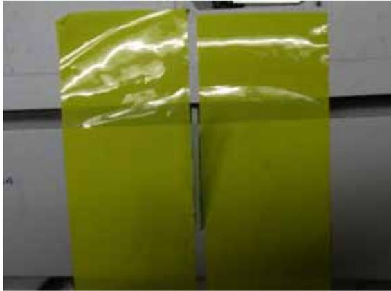
Prepare the area to epoxy the control horn in position by protecting the area with packing tape. Leave minimal area between the slot and the tape to allow a small epoxy fillet to be formed between the control horn and the control surface skin. Apply epoxy by filling the slot with epoxy prior to inserting the control horn, the object is to epoxy the control horn to both the top and bottom surface. A thickening agent such as cut fibers will improve the strength of the bond.
