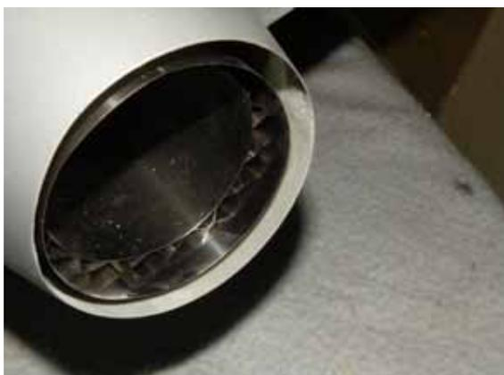
The tailpipe should be inset 5mm from the fuselage opening to improve the flow of
