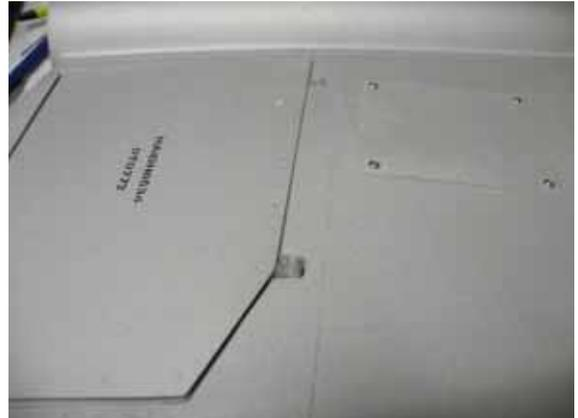
The flap surface fit is very good out of the molds, but the depth of the hinge pocket will be required to be adjusted to attain this flush fit with the hinges installed. Lubricate the hinge pins prior to installation. The hinges can be epoxied in place to the wing and flap at the same time. Carefully position the flap in the pocket as the epoxy cures to assure bind free movement of the flap.
