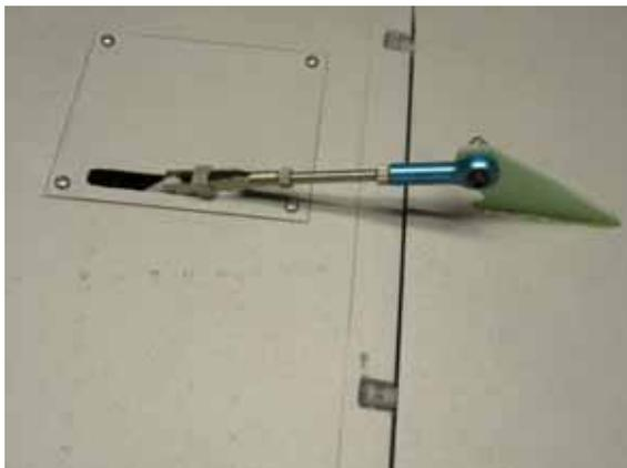
Final appearance of the installed outer flap servo and control linkage, again care must be used to epoxy the control horn to both the upper and lower surface of the flap.
