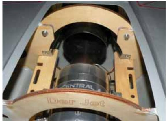
Secure the tailpipe with the provided straps to the aft spar former with wood screws, bend the straps as necessary to properly center the tailpipe to the turbine. Note the tailpipe straps are stainless steel, the use of a sharp drill bit will be necessary to drill through this metal strap.
