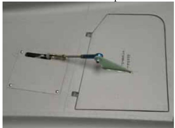
The servo installation is similar to the elevator installation process, again use care to assure the control horn is epoxied in place to both the upper and lower surfaces, trim control horn as required to assure a flush fit.
