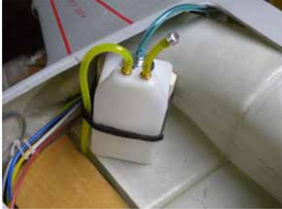
The ECU tray is to be installed behind the inlet under the main hatch. this tray allows for installation of turbine systems, i.e. fuel and gas valves, ECU. This aft tray is a good choice for mounting the air fill valves for the brakes and retracts as it allows topping off the air with removal of the rear top hatch only.
