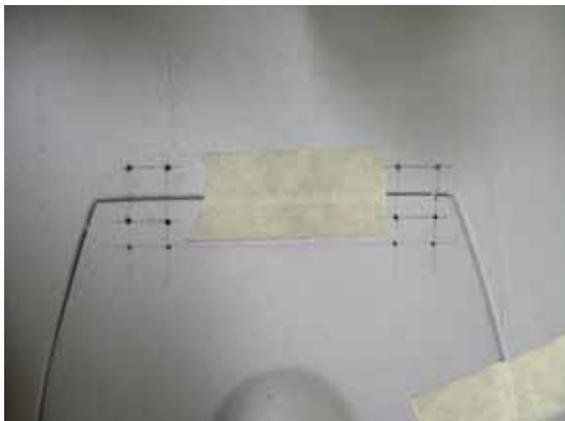
Layout main gear door hinges with the doors taped in proper location. Drill all holes then and install hinges. This will assure a quality fit of the doors to the wing pocket. The front hinge must be installed as far forward as allowed to properly fit the main gear air cylinder later.
