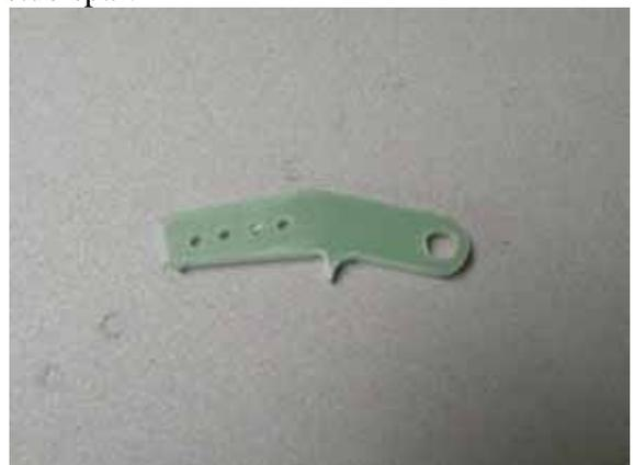
Locate the air brake control horn and drill out for the 3mm dia. linkage bolt. Scuff sand the lower section to improve epoxy adhesion.
