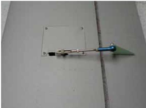
Once the epoxy is dry complete the installation by re-attaching the control linkage to the control horn. Trim the hatch to clear the control arm and linkage, then install the hatch in place with the screws that were removed in the initial step.
