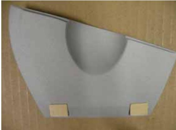
Plywood shims may be required to obtain a flush fit of the door to the wing skin. Make from scrap material if required and sand the thickness to obtain a flush fit by trial and error when screwing the gear door in place.
