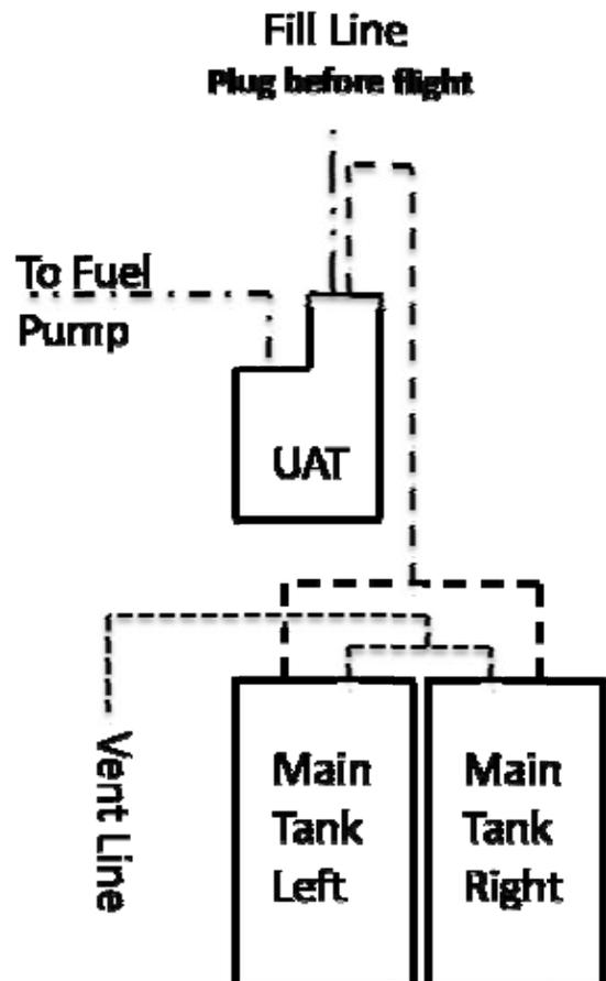
Fuel system setup is to "Y" the main tank pickup lines to the one of the two fittings on the UAT. The vent lines of the two main tanks can be connected with a T fitting and vented to the outside. The 2nd fitting off the
