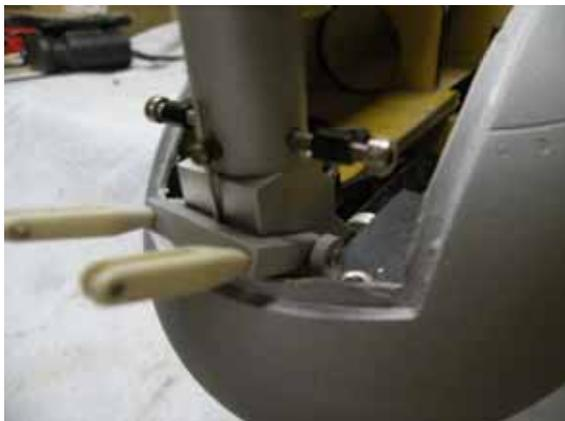
Assure adequate clearance between nose gear cover link rods, nose gear strut and fuselage to allow nose gear to fully lock in down position. It may be necessary to sand some clearance to the fuselage door lip to assure full travel of the nose gear strut to the lock position. *If your model does not have adequate clearance you will need the 8mm thick spacers under the retract unit.*
