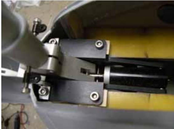
Mount the retract unit with the nose gear cover link rod secured by front bolts. The air line must be connected to the fitting on top side of air cylinder prior to installing nose gear retract. *Note 8mm x 18mm x 55mm spacer plates located under nose gear retract unit for proper spacing on earlier kits.*
