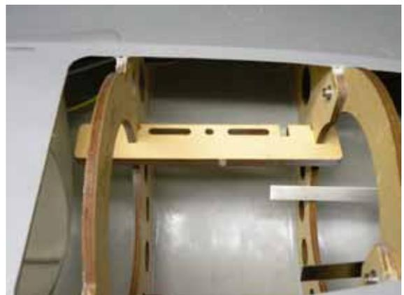
The turbine mounts can be spaced according to your selection of turbines. Shallow slots are provided to allow for small diameter turbines in the 89mm to 93mm diameter size, for larger diameter turbines a set of deeper slots are provided. Epoxy the mounts in place after trial fitting your turbine to assure proper spacing.
